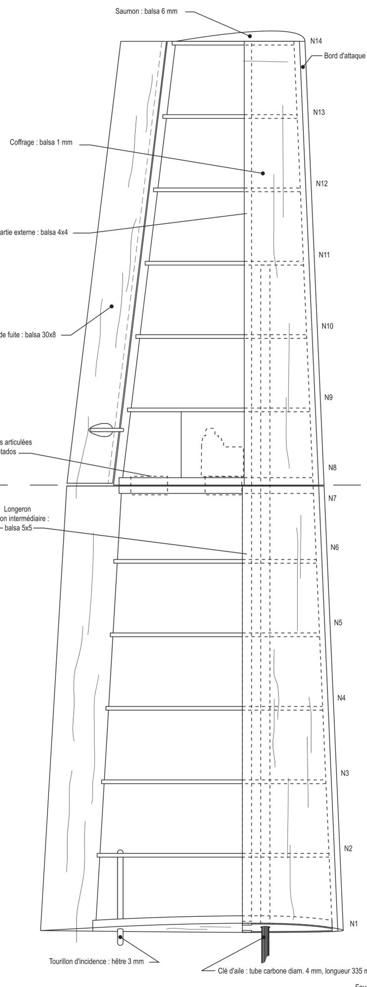
AILE DROITE VUE AVEC COFFRAGE AU BORD D'ATTAQUE DESSUS/DESSOUS
